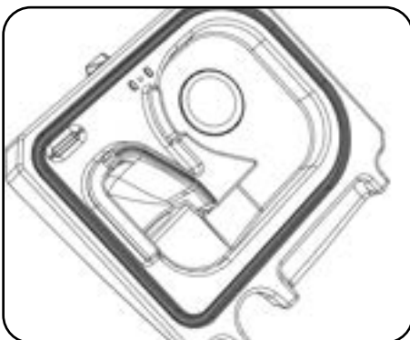
Clean and examine rubber seal during each clean.
