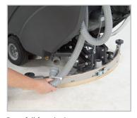
For a full functioning extractor, move the hose to the vacuum shoe inlet and raise the squeegee
